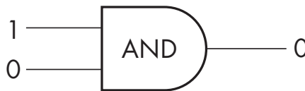
Figure 1.7 An AND logic gate with two inputs and one output. If either of the inputs is 0, the output is 0. If both inputs are 1, the output is 1.
